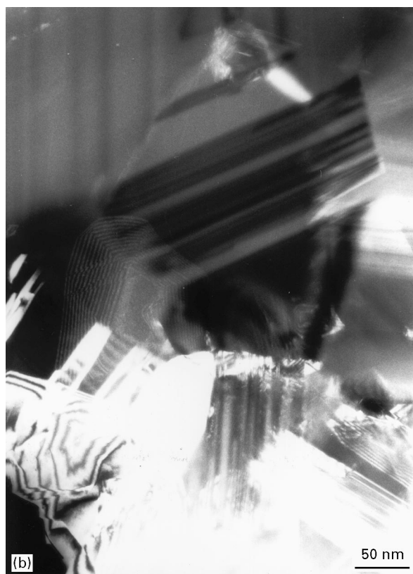
Figure 6 Quasi-stoichiometric 1800°C-pyrolysed SiC fibre; (a) bright field image and (b); dark field image, SiC-(111) reflection.
